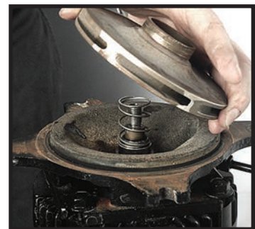
Aligning impeller and spring
